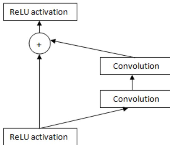
**Figure 1. Block diagram of ResNet**
